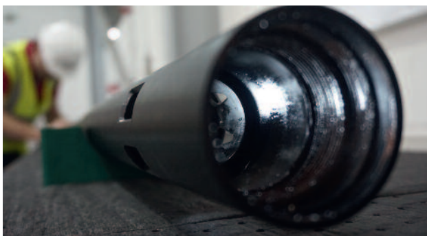
Figure 5. PulseEight technology simplifies operations by removing the need for traditional hydraulic or electric control lines
