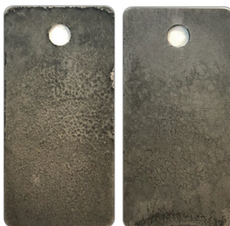
P-110 Alloy in ScaleFix CSD 149°C (300°F) after 6 hours
