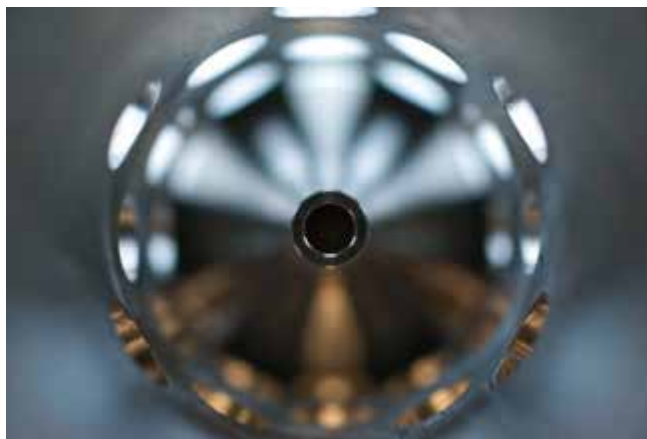
The PT Gauge system uses innovative intelligent pulse technology to choke well flow intermittently so that existing sensors at the wellhead can receive the signals
