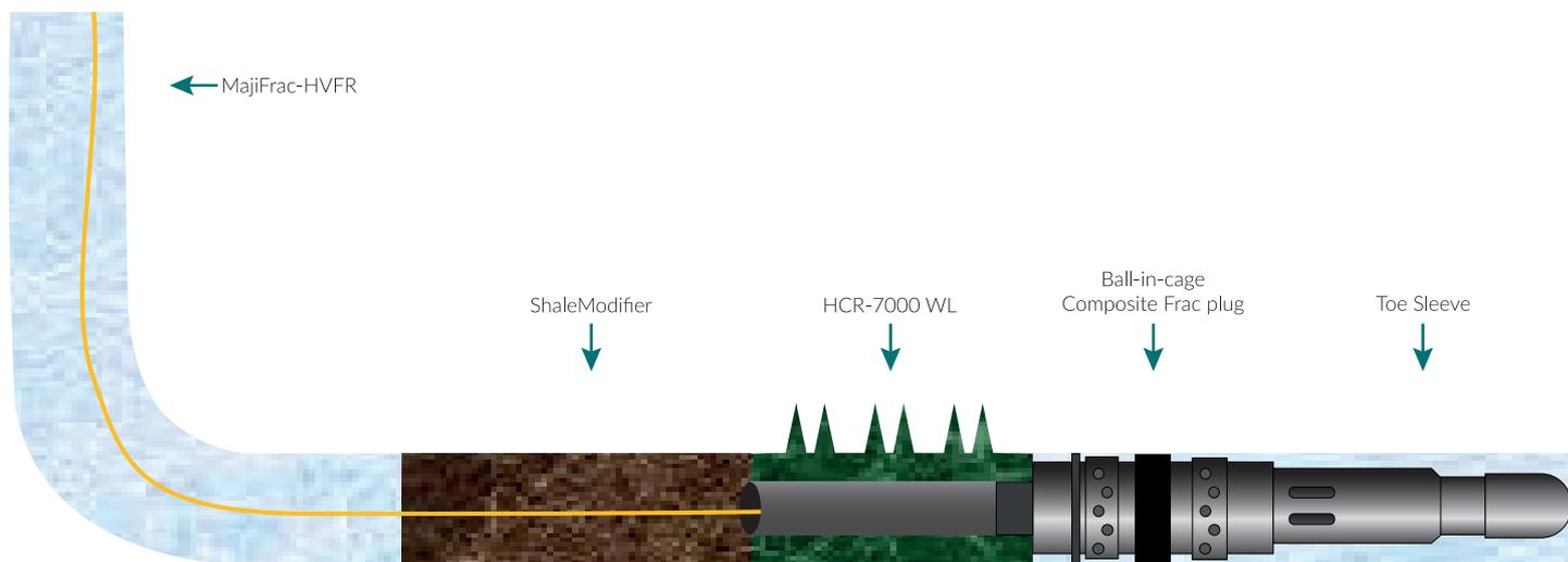
Figure 2: The MajiFrac Plus Solution includes an acid-resistant FracRight fully composite frac plug, a wireline-friendly modified spearhead acid system, ShaleModifier and a range of HVFRs.
