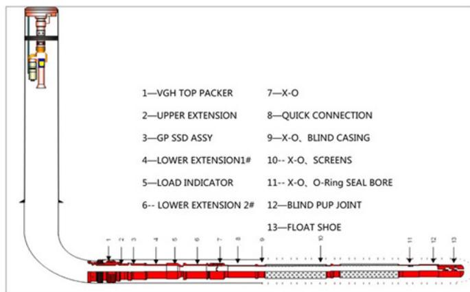
Figure 3: Well C2H completion schematic
