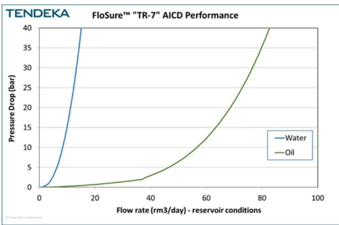
Figure 4: AICD performance curve
