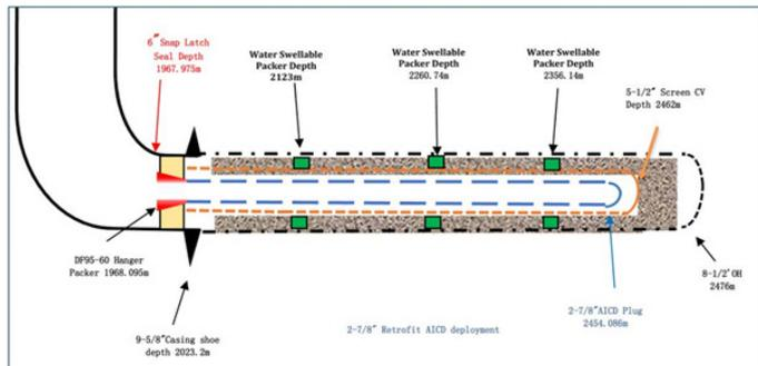
Figure 5: Well C1H completion schematic
