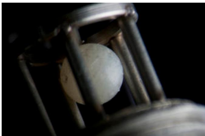
Tendeka's FloCheck valve allows for circulation to the bottom without an inner string. Once production is initiated, the ball simply comes off-seat.
