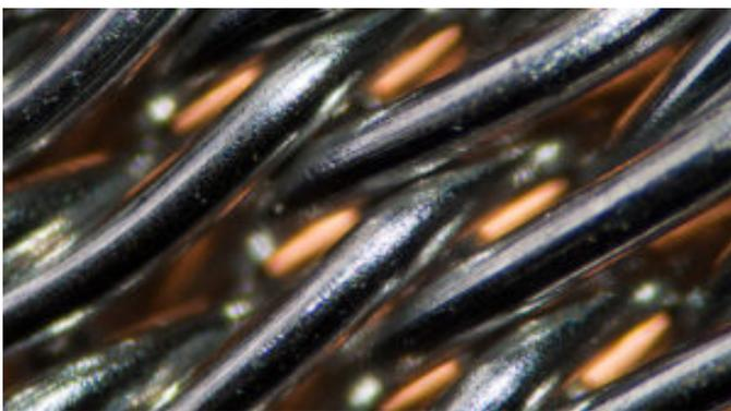
Inflow control devices can be installed as a standalone option or in conjunction with a sand screen such as the FloMax Dutch Weave sand control screen (Image courtesy of Tendeka)
