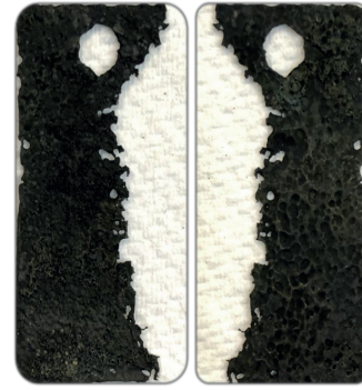
P-110 Alloy in inhibited 15% HCl 300°F Acid blend after 6 hours
