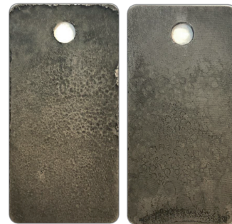
P-110 in 33% HCR-7000-WL Eagleford (300°F) Modified Acid Blend after 6 hours
