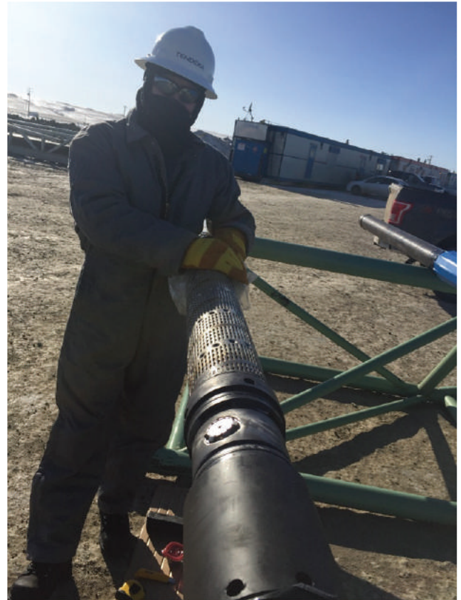
AICD completion being prepared for deployment on site
