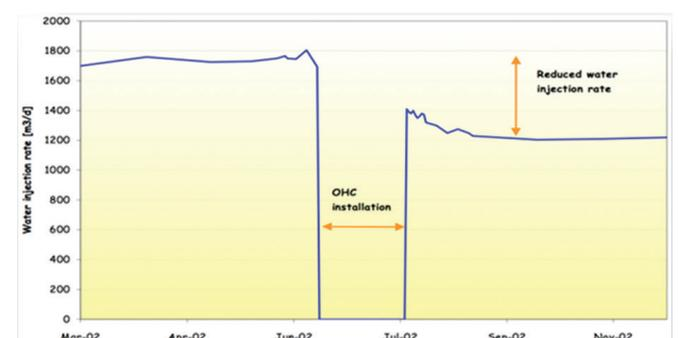
Figure 2 - Water injection rate before and after swellable packer installation
