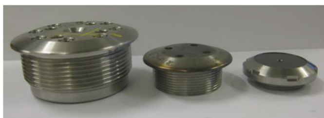
Figure 4: Design evolution of the RCP AICD from original device AR2 (l), with revised fluid path TR7 (m) and with a revised construction TR7-2 (r)
