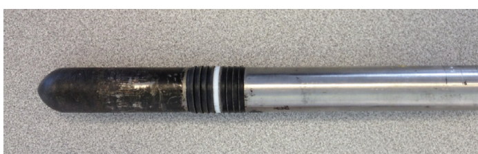
Damaged Gas Lift Valve
