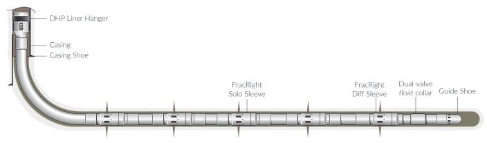
FracRight Solo Sleeve System for Cemented Applications
