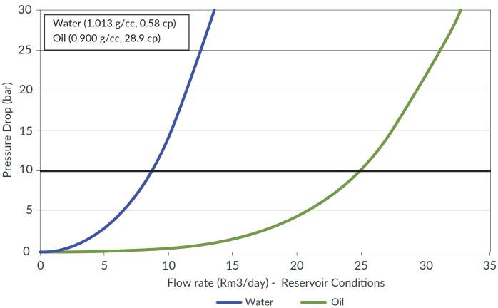
Pressure drop versus flow rate for water and oil is plotted for visualisation of the mobility control imposed by the FloSure AICD. It illustrates flow rate through the valve increasing with 28cp oil compare to water. The mobility ratio between water and heavy is 2.5 times. This implies that water travels faster at similar pressure gradient compare to oil and lead to reduction in water flow at similar pressure drop.
