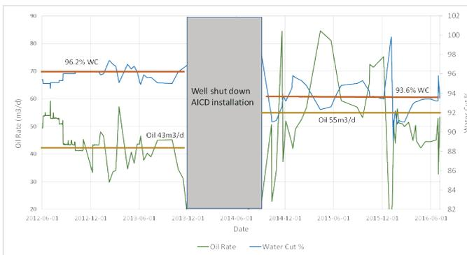
**Figure 2:** AICD oil rate and water cut performance in an existing / retrofit well
