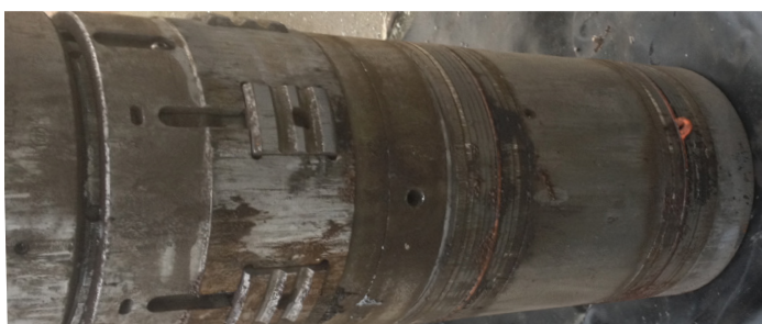
Injection sleeve retrieved from well with Encapsulated O-Rings still intact.
