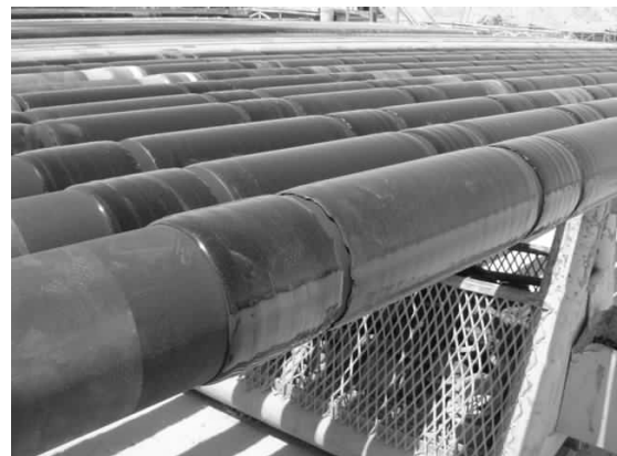
Figure 6: Solid expandable pipe with swelling elastomer elements
